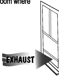
Door or window should be open 4 to 6 inches
