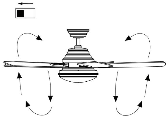
**Cool weather - (Reverse)** An upward airflow moves warm air off of the ceiling. This allows you to set your heating unit on a cooler setting without affecting your comfort.
