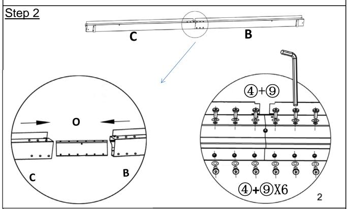
Attach Bar Union(O) between Left Short Beam(B) and Right Short Beam(C) using Bolts(4) and Washers(9) with Allen Key(7).
