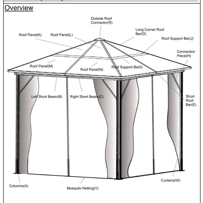
This Gazebo has multiple parts and may require up to 3 hours to assemble. To give you an overview of the Gazebo parts, the above picture is to help you put the various parts into perspective. Please read through the instructions below to familiarise yourself with the parts and steps before assembly.
