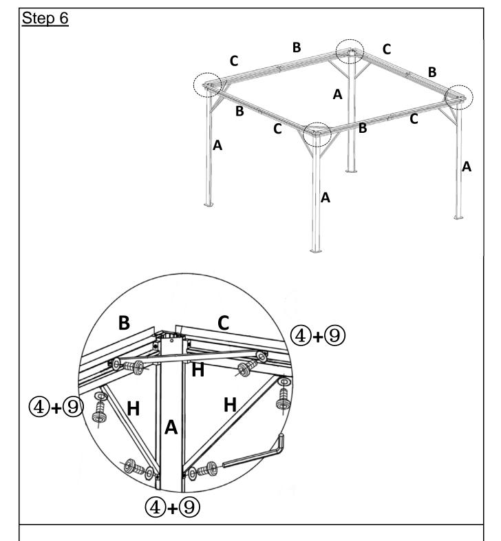
Attach Connection Piece(H) between Left Short Beam(B) and Right Short Beam(C) using Bolts(4) and Washers(9) with Allen Key(7).
