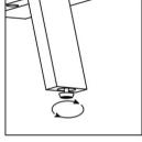
Adjust bottom screw to tighten.
