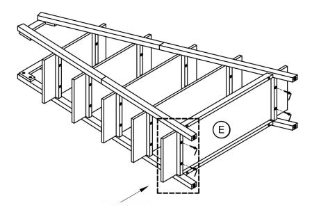
Attach stretcher to frame leg with screw.
