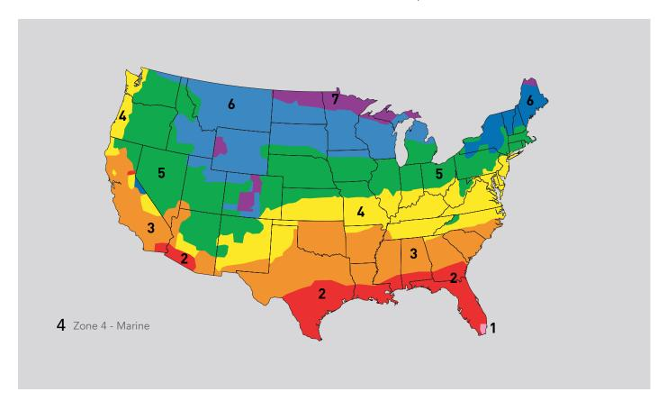
In the northern states and Canada, chances are that building code mandates a vapor control layer be installed on the warm side of the insulation. A vapor control layer in northern climates helps to reduce the moisture diffusion through the wall assembly and through to the drywall.
