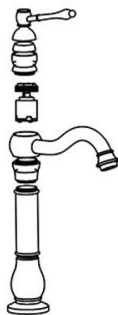
Single-Handle Vessel Sink Faucet Installation
