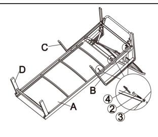
Attach Left Armrest/Leg(B) to Seat (A) using Bolts(②) and Washer ③ with Allen Key ④ as shown above.
