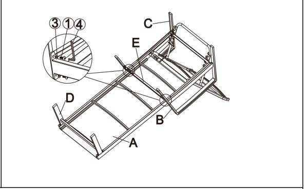
Attach Support Bar (E) to Left Armrest/Leg(B) to Right Armrest/Leg(C) Bolts(1) and Washer 3 with Allen Key 4 as shown above.
