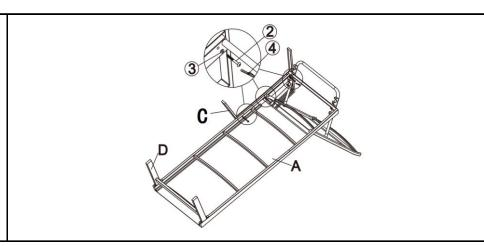
Attach Right Armrest/Leg(C) to Seat (A) using Bolts(2) and Washer(3) with Allen Key(4) as shown above.
