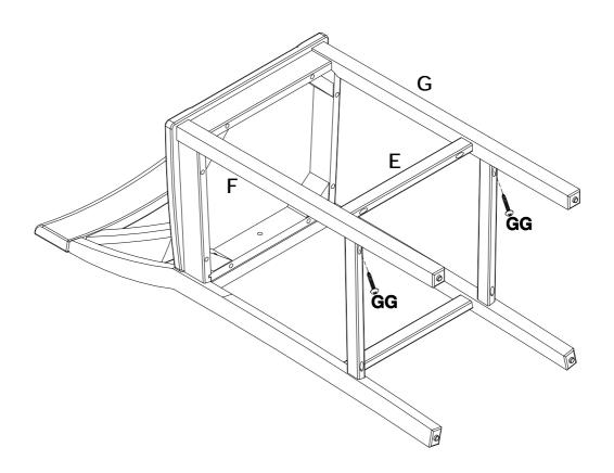
Fix left leg(F) and right leg(G) to seat panel (B) with screw(FF) and washers (CC&BB) by allen key(DD) BBx4 CCx4
