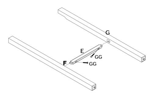
5 Attach left leg(F) to left side rail (C)and right leg(G) to right side rail (D) with screw(GG).
