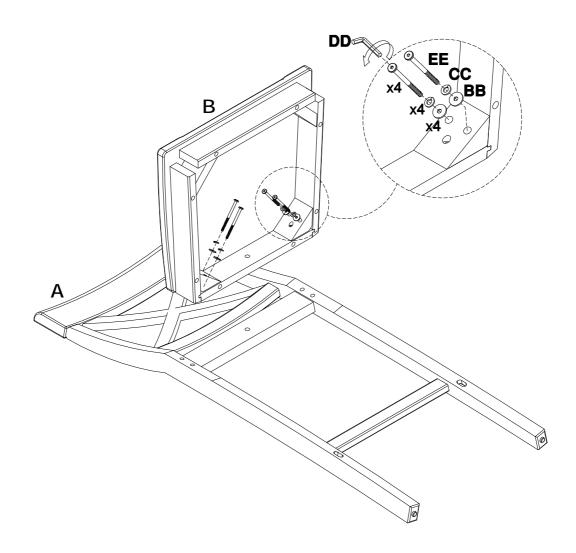
2 Use allen key(DD) to drive screw(AA) with washers (CC&BB)as shown,make sure the seat panel(B) and backrest frame(A) more stable.
