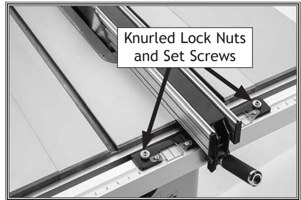
Figure 111. Location of lock nuts and set screws for adjusting fence squareness and height.
