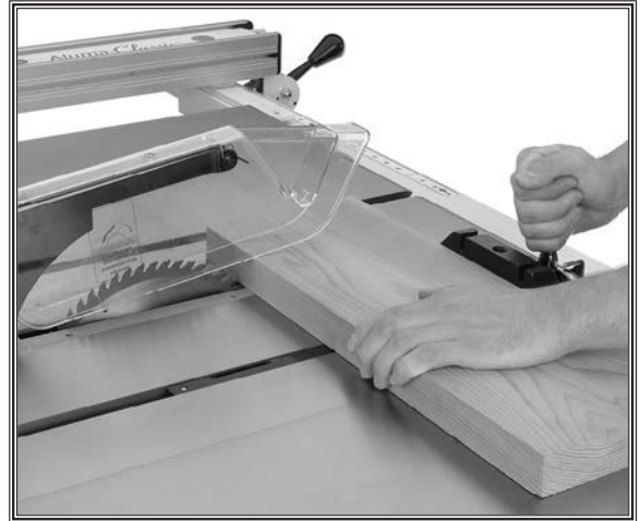
Figure 56. Typical crosscutting operation.
