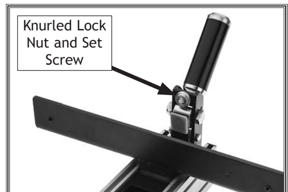
Figure 116. Set screw for adjusting fence handle clamping pressure.
