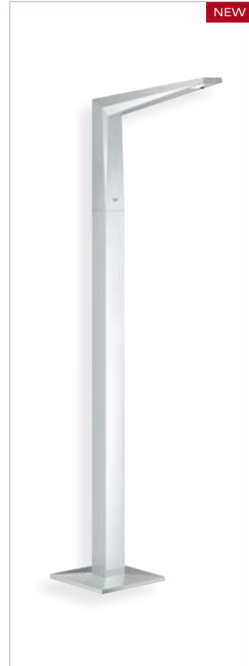
13 301 000 Floorstanding tub spout 3 37 13 / 16 "–40 15 / 16 "(960–1040mm) product height 10 5 / 8 " (270mm) spout/aerator reach
