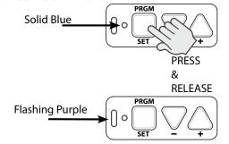
**NOTE:** The openers LEARN LED will time out in 30 seconds. Programming must be completed within 30 seconds.
