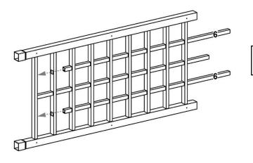
Insert 55" vertical rails (part 6) through remaining holes in cross rails.
