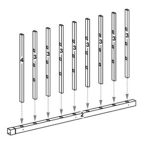
Lay out right post (part 2). Starting at bottom (flared end), insert bottom cross rail (part 4) and center cross rails (part 3).
