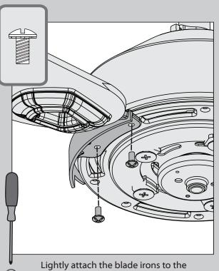
motor with screws found in the X hardware bag, then securely tighten after both screws are attached.
