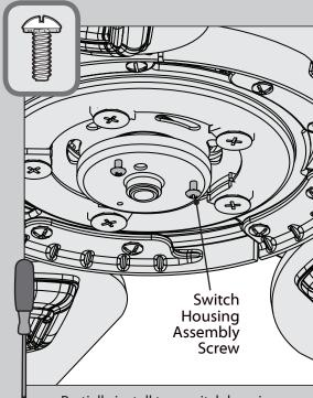
Partially install two switch housing assembly screws ,found in the == hardware bag, into the motor housing as shown. It does not matter which two screw holes you choose.
