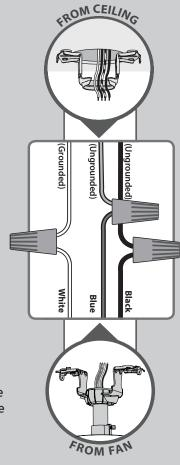
Turn the splices upward and push them carefully back through the hanger bracket into the outlet box. Spread the wires apart, with the grounded wires on one side of Refer to CAUTION c.1 on pg. 2 the outlet box and the ungrounded wires on the other side of the outlet box.
