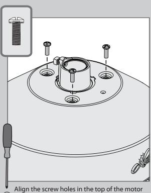
housing with the screw holes in the motor assembly. Install the three motor housing screws, found in the hardware bag.
