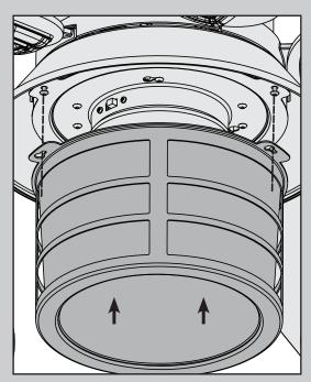
Align the keyhole slots in the globe assembly with the partially installed screws in the light kit assembly.
