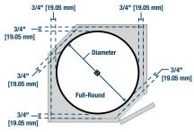
Dimensions shown are recommended minimum cabinet dimensions and clearances.
