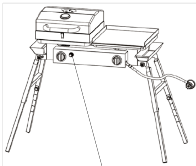
Electronic Ignition Button. Unscrew, insert AA Battery, replace button
