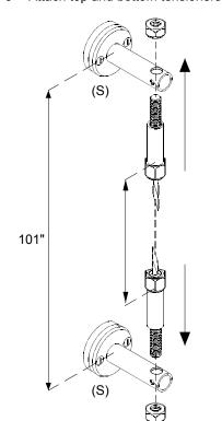
6 Tension the cables using nuts untill the cable is straight
