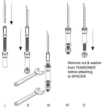
Remove nut & washer from TENSIONER before attaching the cable.
