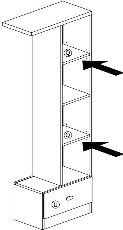
*\*Place adjust panels (Q) into cabinet as shown.*
