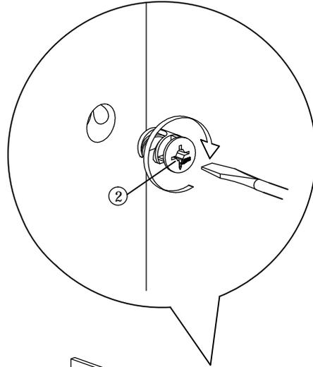
*\*Assemble (N) panel secure with Minifix as shown.*
