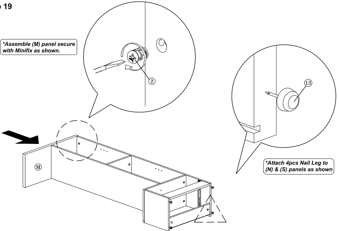
*\*Attach 4pcs Nail Leg to (N) & (S) panels as shown*
