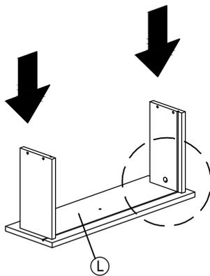
*\*Assemble drawer side panels, secure with Minifix as shown.*
