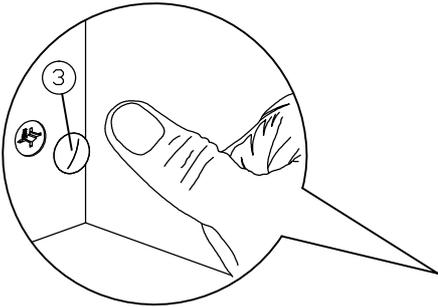
**\*Attach 2pcs Minifix Cap to both drawer side panels as shown.**
