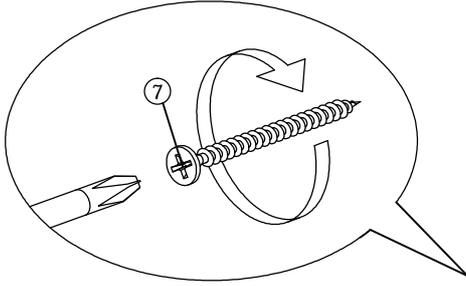
**\*Insert drawer back, secure with screw as shown.**
