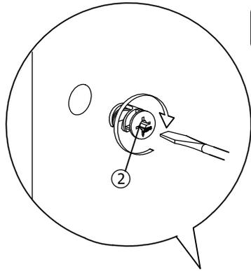
*\*Assemble (E) panel secure with Minifix as shown.*
