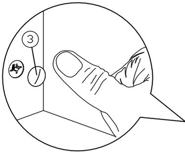
**\*Attach 2pcs Minifix Cap to both drawer side panels as shown.**
