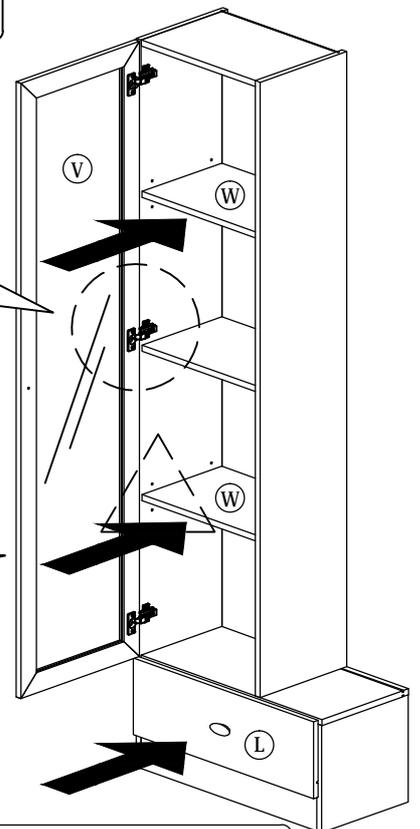
**\*Place drawer (L) & adjust panels (W) into cabinet as shown.**
