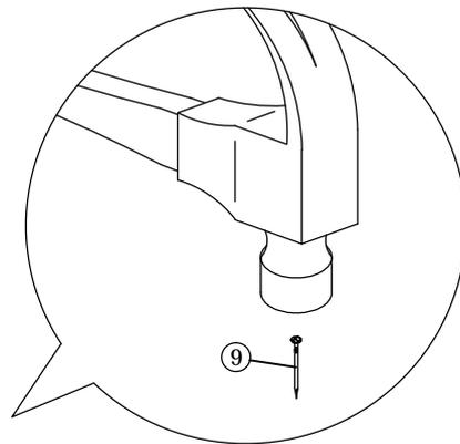
*\*Insert back panel, secure with Nail as shown.*
