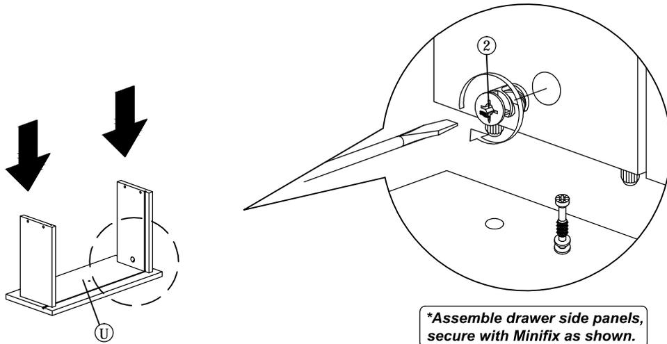
*\*Assemble drawer side panels, secure with Minifix as shown.*
