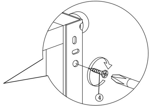
**\*Install Drawer Slide with screw as shown.**
