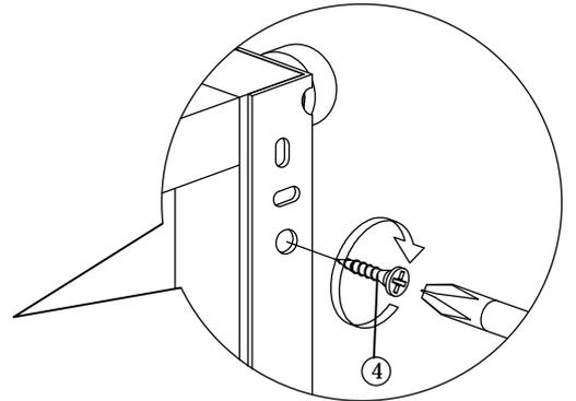
**\*Install Drawer Slide with screw as shown.**
