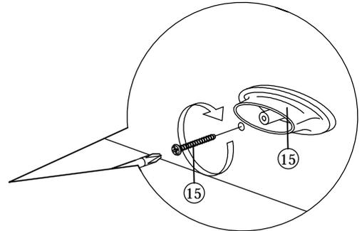
**\*Install Handle to drawer front with screw as shown.**
