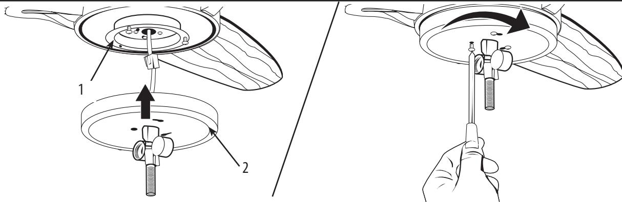
Attach the light kit (2) to the light kit plate (1) by placing the keyslot holes from the light kit onto the two protruding screw heads from the light kit plate. Twist the light kit clockwise until the screwheads engage the keyslots. Install the screw removed from light kit plate (step 20) into the closed hole in the light kit. Tighten all screws to complete attachment of the light kit.
