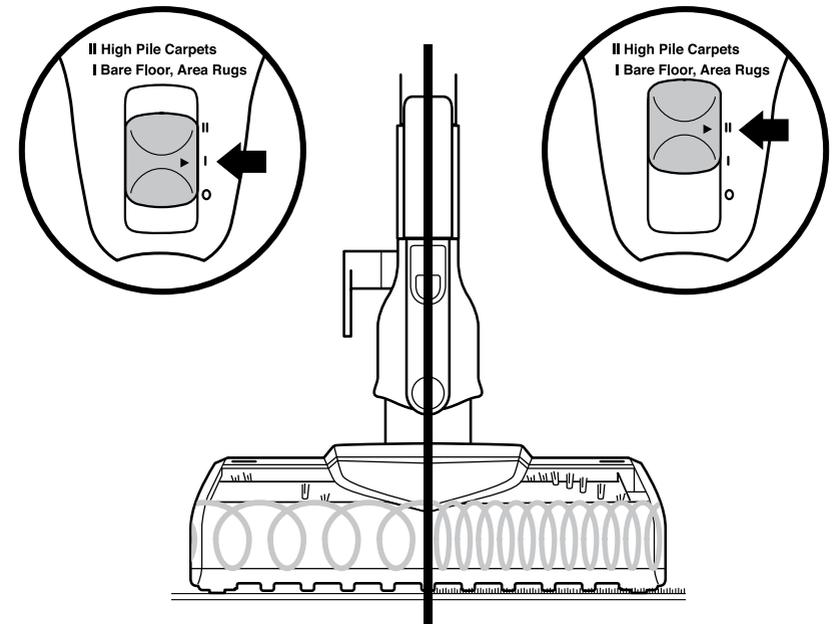
The Rocket™ has a 2-speed Power slider switch on the handle to select the speed of the brushroll. Slide the switch to appropriate speed setting (I or II) and start cleaning.
