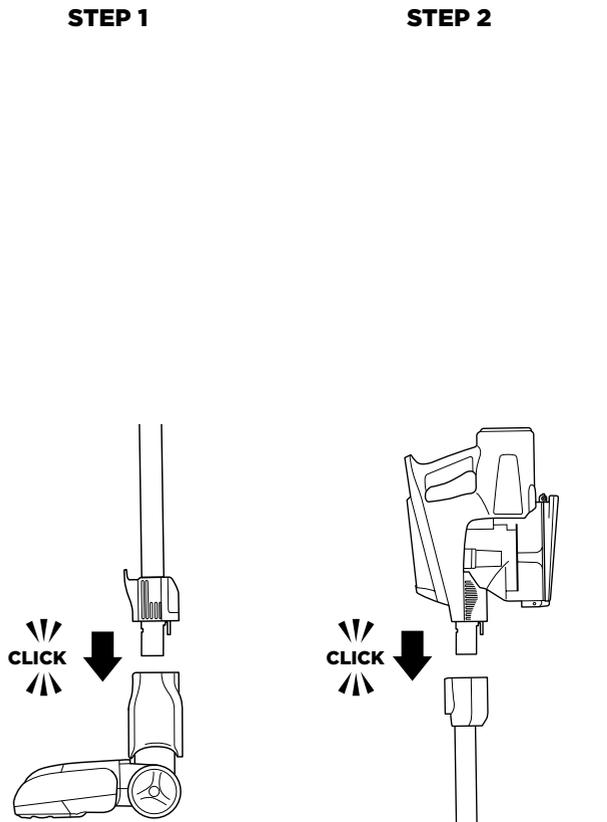
**1** Insert the wand into the motorized floor nozzle connector until you hear a click.
