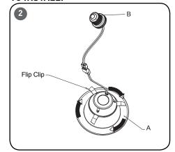
STEP 1: Carefully rotate the "Flip Clips" clockwise until the clips are fully-deployed. See Figure 2.
