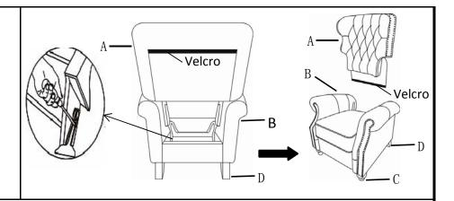
Disassembly Note:Open the flap on the Chair Backrest(A),use a screwdriver(Don't use fingers) pressing outward on the metal ear on the preattached Metal Bracket on one side of the Chair Base(B),with assistance of you adult partner to keep the Chair Base(B) in place, pull out the Chair Backrest(A) upward at the same time,repeat the same step for another side. Then the Chair Backrest(A) can be taken out.
