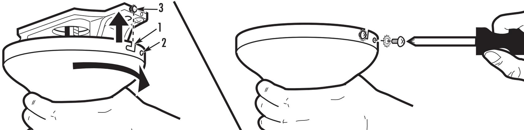
The canopy has two mating slots (1) and two mating holes (2). Position both slots on canopy directly under and in line with two screws in the mounting bracket (3). Lift the canopy, allowing the two screws to slide into the mating slots. Rotate the canopy clockwise until both screws from the mounting bracket drop into the slot recesses. Tighten screws securely. Install two screws and star washers into the mating holes of the canopy and tighten to secure the canopy to the mounting bracket.
