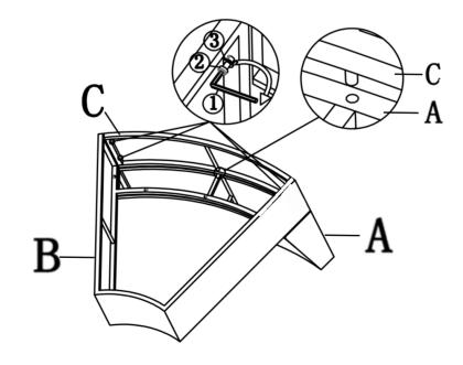
Align the iron dowel of Seat Back Board(C) to mounting position of Seat Board(A). Attach the Seat Back Board(C) to Backrest(B) and Seat Board(A) using Bolts(②) and Washers(③) with Allen Key(①) as shown above.
