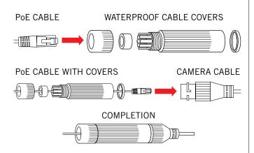
Insert one end of the PoE cable into the cable covers as shown in the image above. Connect the covered end of the PoE cable to the cameras' power cable.
