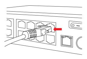
Input the other end of the PoE cable into an open PoE port on the back of the NVR.
