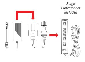
Plug the NVR power adapter into a surge protector or Uninterruptible Power Supply (UPS).
