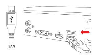
3 Plug the USB mouse into the USB port on the back of the NVR.
