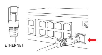
Plug one end of the included Ethernet cable into the LAN port on the back of the NVR.
