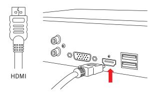
Plug one end of the included HDMI cable into the HDMI port on the back of the NVR.
