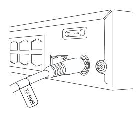
8 Connect the NVR power adapter to the Power Input on the rear of the NVR.
