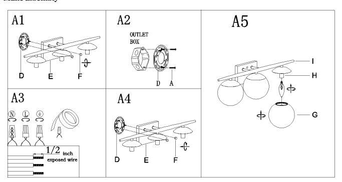
Step A1: Unscrew the threaded ball(F) from the back plate(E) then gently remove the mounting plate (D).
