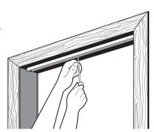
the track. Do not fully tighten. (Tape may be used to hold the track in place while you mark and drill.)
