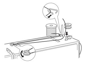
In order to ensure correct bobbin winding, follow the above diagram for correct threading. Use both hands to thread machine around the guide for correct tension.
