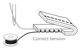
Conversely, if the thread is looping on top, make sure the bobbin thread is coming off the bobbin counterclockwise and that the thread is securely threaded in the bobbin tension guide.
