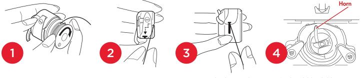
Before inserting the bobbin into the bobbin case, hold the bobbin in your hand and make sure that the thread is coming off the bobbin in a counterclockwise direction (it should look like a "P"). This will allow the bobbin thread to move correctly and to stay lodged in the bobbin tension guide.
