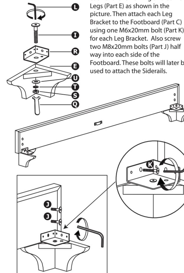
Attach one Leg Bracket (Part R) to each of the remaining two Corner Legs (Part E) as shown in the picture. Then attach each Leg Bracket to the Footboard (Part C) using one M6x20mm bolt (Part K) for each Leg Bracket. Also screw two M8x20mm bolts (Part J) half way into each side of the Footboard. These bolts will later be used to attach the Siderails.
