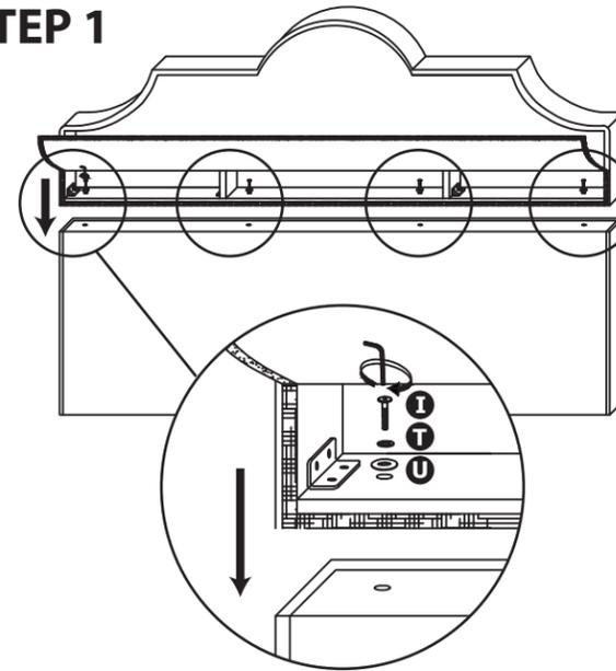
Undo the Velcro and pull the cover off on the back of the Headboard Top (Part A). Assemble the Headboard by attaching the Headboard Top (Part A) to the Headboard Bottom (Part B) using four M8x40mm bolts (Part I), four spring washers (Part T), and four flat washers (Part U).
