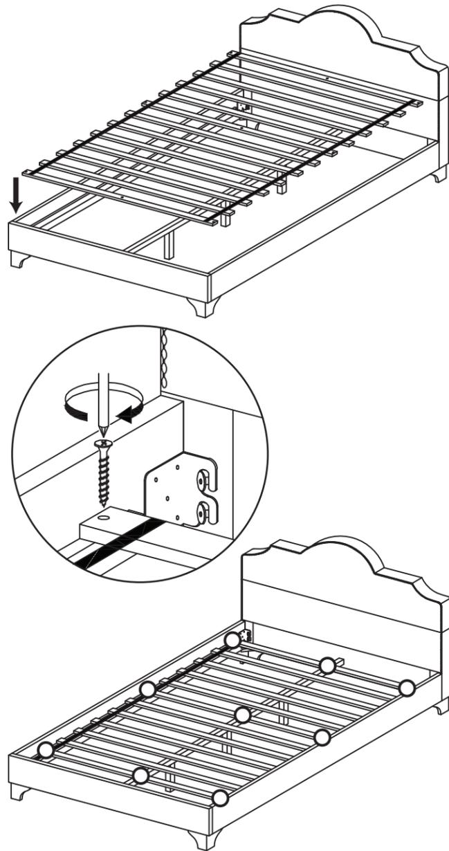
Roll out the Wood Slat System (Part H) and secure it in place with 9 38mm screws (Part N) using the pre-drilled holes and a phillips screwdriver.
