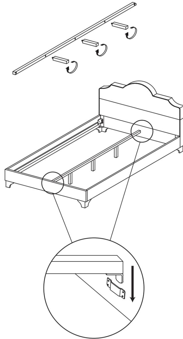
Screw the Center Legs (Part G) into the Center Support (Part F) before inserting the Center Support into the brackets on the Headboard and Footboard.
