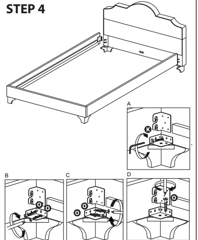
Hang the Siderails (Part D) from the bolts you screwed half way into the Headboard and Footboard in Steps 2 and 3. Then tighten the bolts. Next, finish installing the Leg Brackets (Part R) using the small hex key (Part M) as shown in Step A and using a phillips screwdriver as shown in Steps B, C and D.
