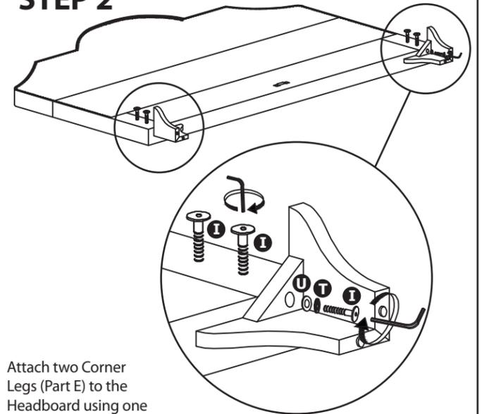
Attach two Corner Legs (Part E) to the Headboard using one M8x40mm bolt (Part I), one spring washer (Part T) and one flat washer (Part U) for each Corner Leg. Also screw two M8x40mm bolts (Part I) half way into each side of the Headboard. These bolts will later be used to attach the Siderails.
