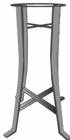
Attach metal ring to frame.
