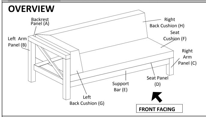
This Left Chair has multiple parts and may require up to 30 minutes to assemble. To give you an overview of the Left Chair parts, the above picture is to help you put the various parts into perspective. Please read through the instructions herebelow to familiarise the parts and steps before assembly.
