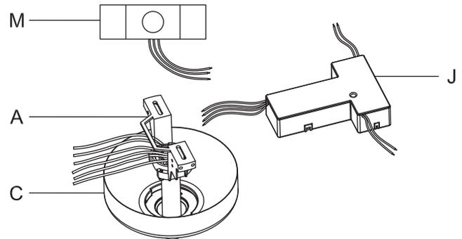
Insert the receiver (J) into the mounting bracket (A) with the flat side of the receiver (J) facing the ceiling.
