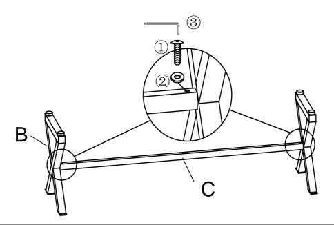
Attach Leg with pre-attached Levellers(B) and Leg Support(C) with Bolts(1) and Washers(2) by Allen Wrench(3).
