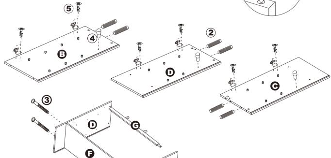
use 8 allen key to fasten allen-head wood screw
