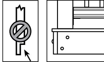
Do not notch the 4x4 railing posts. Notching will reduce the strength of the post and could result in railing collapse or failure. Determine the positions of the rail posts by measuring the runs of the project and placing the posts at the desired spacing.
