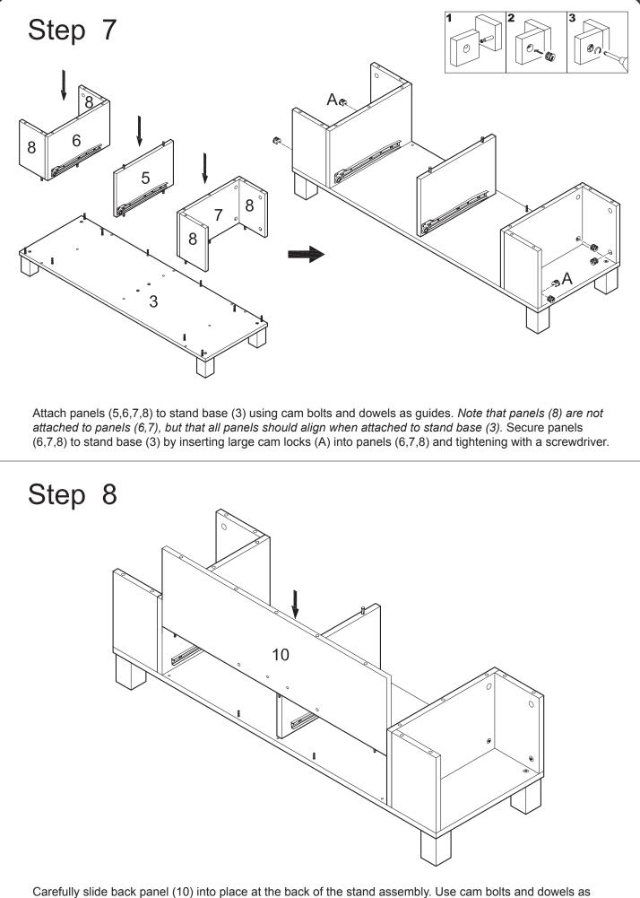
Carefully slide back panel (10) into place at the back of the stand assembly. Use cam bolts and dowels as guides.
