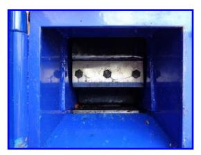
• Rotate the drum until the blade is visible like the above photo. You can rotate the drum by pulling the starter cord but can be rotated by hand (wearing gloves) more precisely. Remove the three bolts holding the blade and remove. Rotate the blade, using the other cutting surface or replace the blade. Torque bolts to 37 ft/lbs. Use blue Loctite on clean threads.
