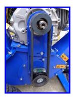
• Loosen (4) <u>engine plate</u> hold down bolts (not the engine bolts ).
