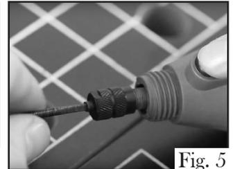
4. Insert the inner core of the flex shaft into the collet nut and collet (Fig. 5). Make sure that the golden metal ring is pressed tightly against the collet nut (Fig. 6). Press down on the spindle lock button, and fully tighten the collet nut with the included wrench.
