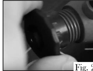
2. Take the flex shaft and slide the inner core out about 2 to 3 inches (Fig. 3).
