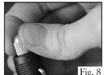
6. Once secured, take the other end of the flex shaft. Find the L-shaped tool and insert it into the hole on the side of the flex shaft handle to prevent the flex shaft spindle from rotating (Fig. 8).
