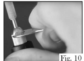
8. Install the collet and collet nut and fully insert the rotary bit into the center hole through the collet (see page 10). Use the included wrench to fully tighten the collet nut and ensure that the bit is properly secured to the flex shaft (Fig. 10).
