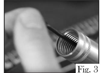
3. Loosen the collet nut on the rotary tool by pressing down on the spindle lock button and unscrewing the collet nut (Fig. 4). Use the 1/8 in. collet for attaching the flex shaft.
