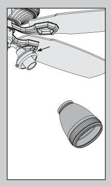
To install the shade, first loosen the thumb screws. Raise the shade to the light fixture. Tighten all thumbscrews securely.
