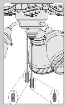
The fan pull chain controls the speed: from high to off.
