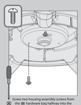
motor housing. It does not matter which
