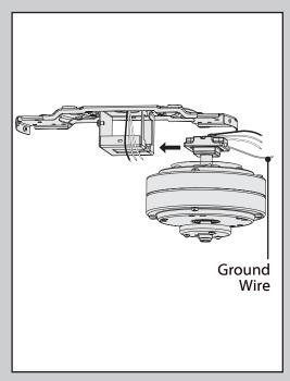
While holding the wires out of the way, lift the motor assembly and place the square hanger into the opening in the ceiling bracket. Be sure the ground wire attached to the hanger faces out of the large opening in the ceiling bracket.
