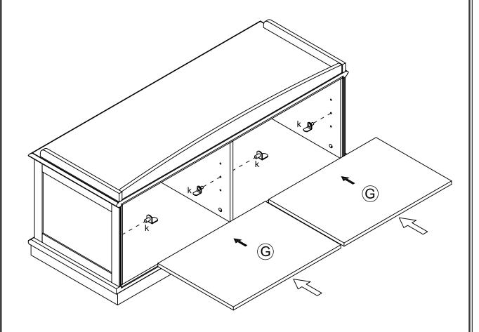
• INSERT THE SHELF PIN (k) IN DESIRED POSITION AND PLACE THE ADJUSTABLE SHELF (G) ABOVE THE SHELF PIN (k).
