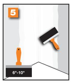
**Skim Coat** Apply a thinner third coat of drywall joint compound to each side, feathered 10" - 12". Allow to dry.
