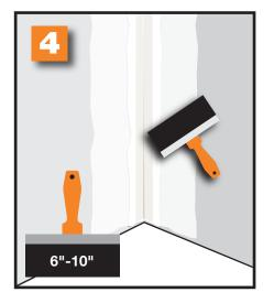
**Top Coat Mud** Using a 6"- 10" drywall taping knife, apply a top coat of drywall joint compound to each side. Feather the compound 8" - 10" from the corner. Allow to dry.
