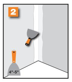
Apply Mud Thin Joint Compound with water. Apply a generous, uniform layer 2" on both sides.
