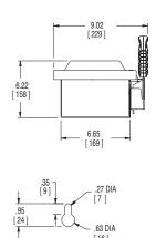
No knockouts in the enclosures. Dimensions shown in inches and millimeters (). Dimension shown accurate to  $\pm \frac{1}{8}$  inch.
