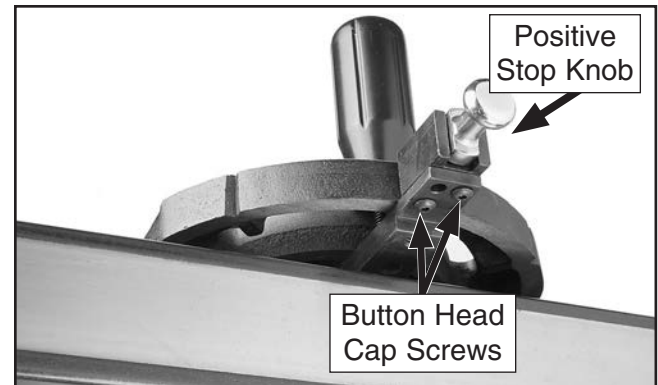
Figure 123. Screws for adjusting miter gauge body.
