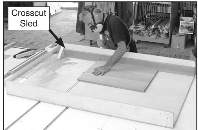
Figure 90. Example of crosscut sled.
