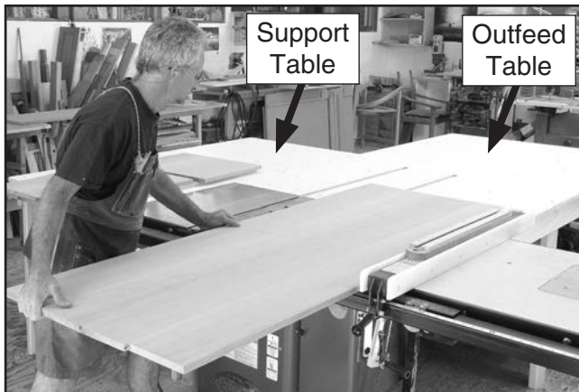
Figure 89. Example of outfeed & support tables.
