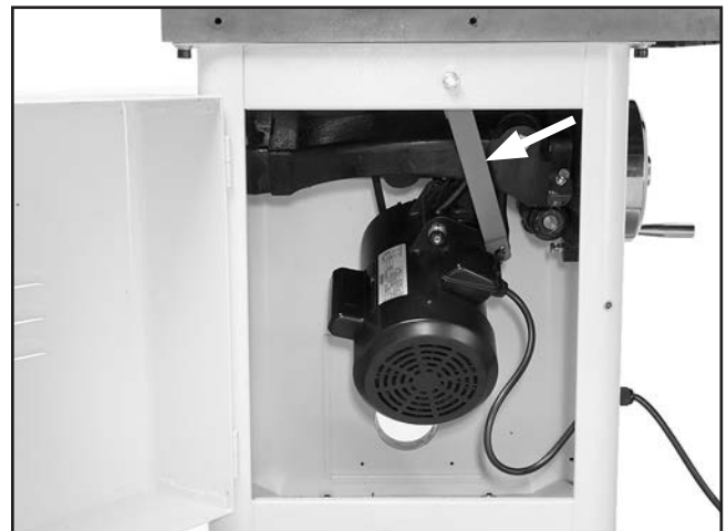
Figure 13. Shipping brace location.
