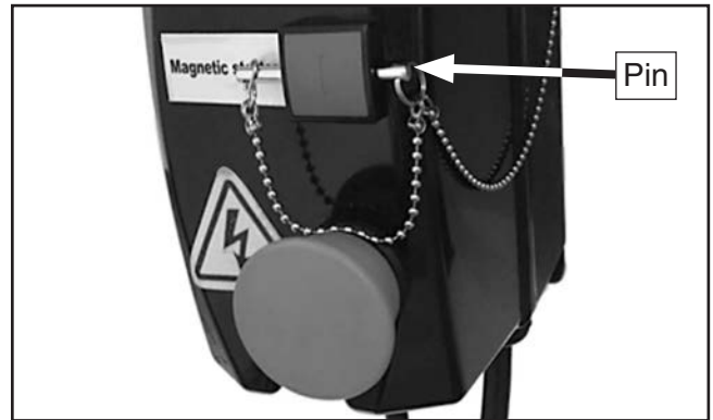
Figure 38. Switch disabling pin inserted into ON button.
