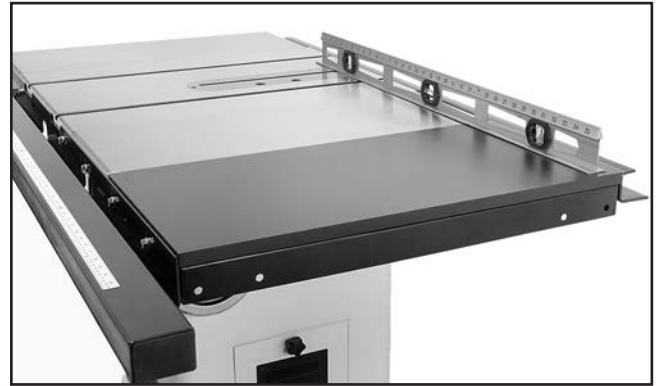
Figure 24. Adjusting Model G0690 extension table flush with extension wing and table.
