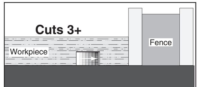
Figure 62. Additional single blade dado cuts.
