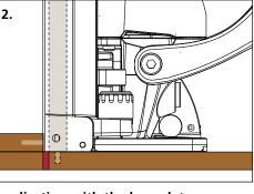
Application with the baseplate The dividing panel (moved by 4 mm) serves as application surface
