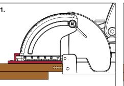
Application with the swivelling front With the 4 mm spacer for 12 mm dividing panel (groove in the center)
