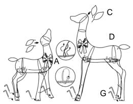
Step 4. Insert both Ears (C) into the matching holes at the top of Head (B). Attach the Bow Tie (A) to the Body (D). (FIG.2)
