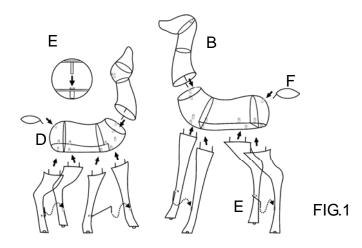
Step 1. Insert the rods at the top of the Legs (E) into the holes on the underside of the Bodies (D). (FIG.1)
