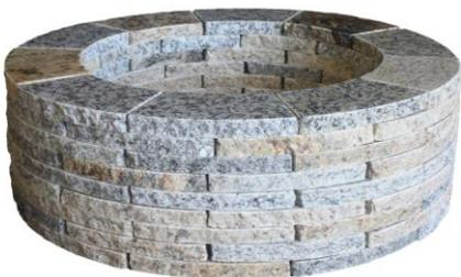
**Step 4:** Install the remaining 7 rows. Place the blocks in the same manner as Step 2, each row staggering the joints of the blocks below. After making any adjustments to each row, remove one block at a time and glue to the two blocks below using quarter-sized dabs of concrete adhesive. Installation is complete – Enjoy!
