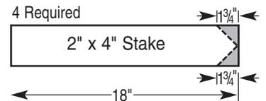
**Note:** For stake angle cut, measure 1 3/4" from straight cut. Draw a line from measurement to center of straight cut.
