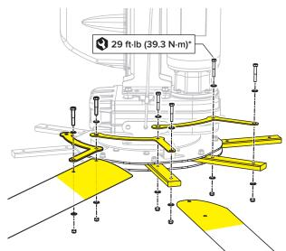
\*If the hardware is stainless steel, ensure bolts are torqued to **10 ft·lb (13.6 N·m)**.
