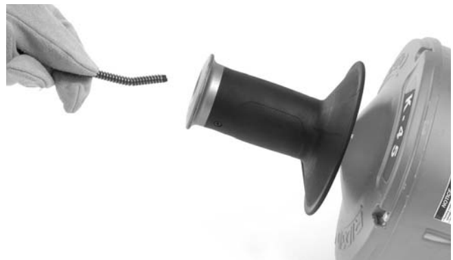
Figure 17 – Loading Cable Without Changing Inner Drum
