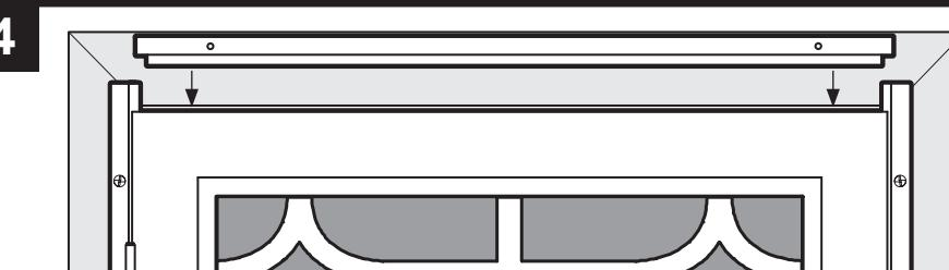
Place the top header jamb (**C**) above the door and between the two side jambs. Spacing should be equal, from left to right, above the door and be similar to spacing determined in **Step 3**. Mark the location of the mounting holes. Set the jamb aside and, where marked, pre-drill 3/16" holes. Return jamb to position and fasten to house using the provided one-way screws (**G**).
