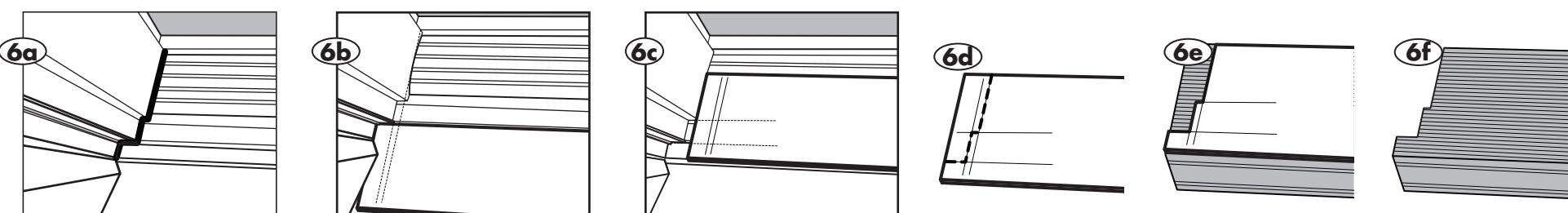
Using a box knife cut template to shape of molding and trim revealed by the markings (**6d**). Test fit the template. (It should lay across the bottom bar, with the front edge flush with the front edge of the bottom bar and fit in and around the corners of the existing molding and trim.)
