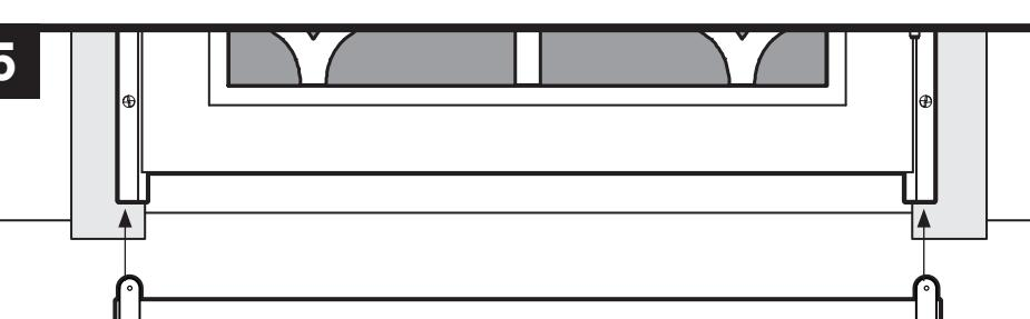
Place bottom bar (**D**) beneath the side jambs. Both ends should reach the outer edge of the side jambs. Hold in place and use 5/32" drill bit to pre-drill holes for mounting screws. Attach bottom bar to each side jamb using the provided screws (**H**).
