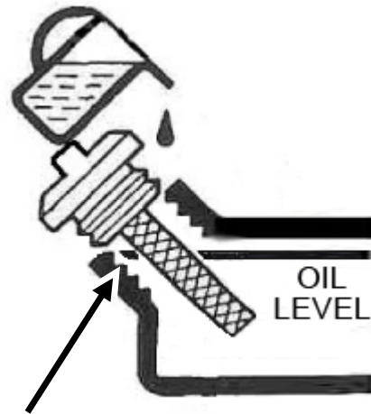
Figure 2 - Add Oil To TOP Of Threads
